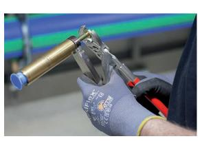
5. Remove the drilling residues from the core bit using a special tool
